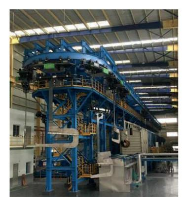
Fully automatic ring track tunnel pickling and coating system for C-steel bundles with a ZLĎ
