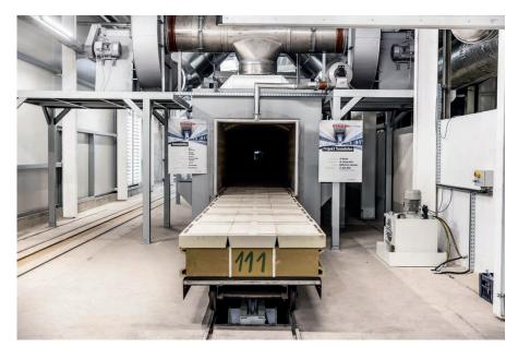
Caption: Empty kiln cars will be driven into the new tunnel kiln during the heating phase
